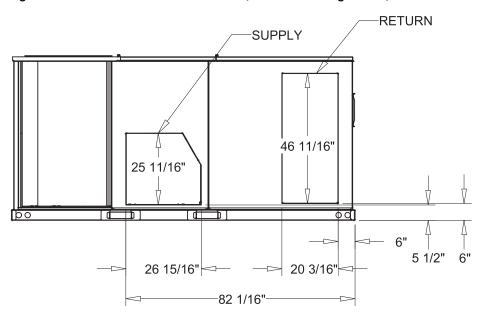
Figure 6. Roof curb -15-22 tons standard efficiency
