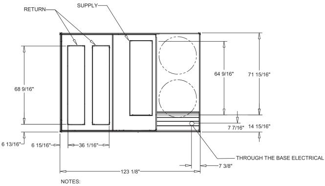
Figure 4. Cooling with optional electrical heat units — plan view — 15-22 tons standard efficiency
