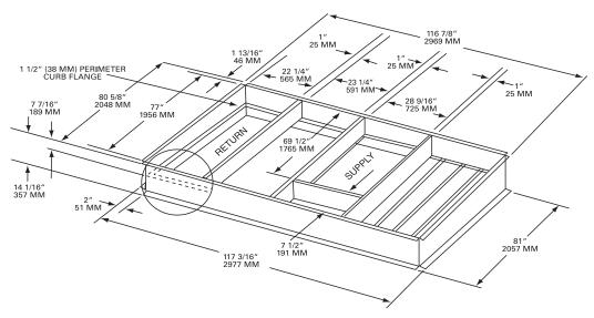
Figure 7. Downflow duct connections—field fabricated 15-22 tons standard efficiency
