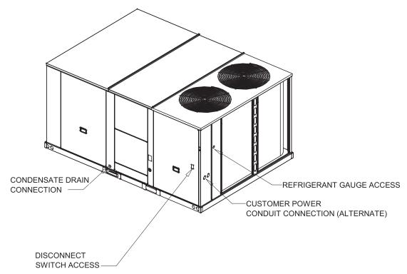
Figure 2. Cooling with optional electrical heat units — overview
