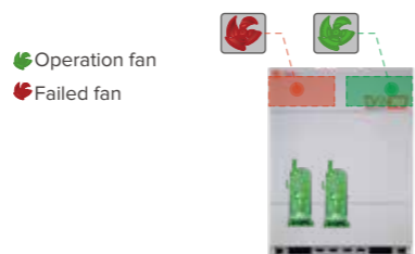
Automatic backup operation of another fan in case of failure of one fan
